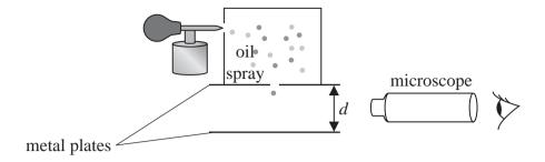
Negatively charged oil drops are sprayed into a region above two parallel metal plates. The plates are separated by a distance d. The oil drops are allowed to enter the region between the two plates.
