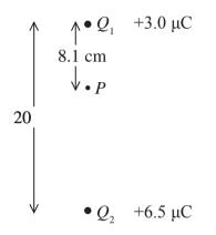
At point P, a distance 8.1 cm from  $Q_1$ , the electric field strength is approximately zero.
