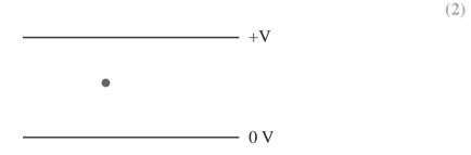
(b) V is gradually increased. At a particular value of V, the oil drop stops falling and remains stationary between the plates.
